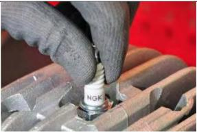
Insert the coil cable into the rubber plug cup so it is tight.
