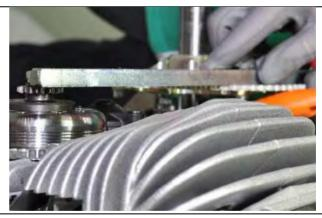
To adjust chain tension, move the engine ahead until the proper tension is reached. Proper tension is around 1 cm. of free up and down movements.
