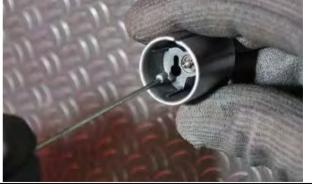
Hook the lead nut in the slide by moving it aside of the center.
