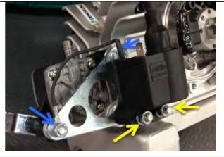
Insert "stop" cable end coming from the ignition into the coil plug.
