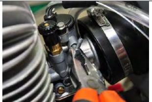
Insert the plastic tube provided on to each one of the carburettor overflow elbows.
