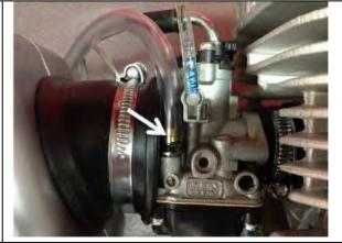
Insert the air tube into the intake silencer and then place the plastic stone guard on top of the air tube.
