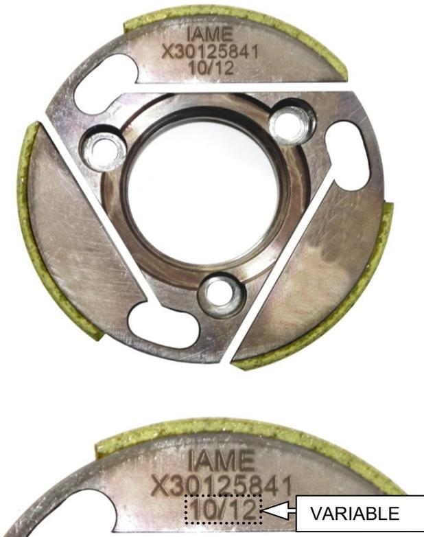
CLUTCH DRUM IDENTIFICATION MARKING
