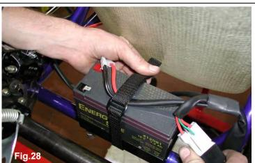
**3.8.6** FIX THE STARTER RELAY TO THE FIXING STRAP BY MEANS OF A CLAMP, OR FIX IT TO THE BATTERY SUPPORT WITH THE BIADHESIVE TAPE (SEE FIG.29).
