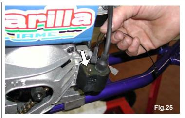
**3.8.3** CONNECT THE SECOND TERMINAL OF THE IGNITION STATOR TO THE "MALE" CONNECTOR OF THE HARNESS (SEE FIG.26).
