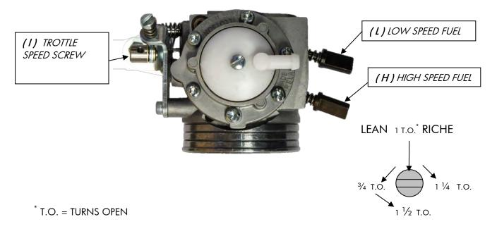
Normally the correct setting of the mixture screws, after engine run-in, is the following:
