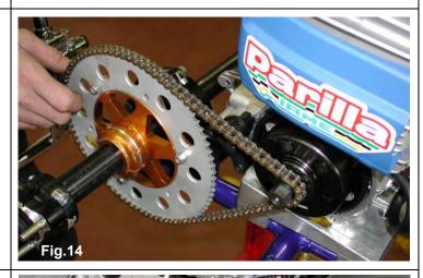
**3.5.4** MOVE THE ENGINE ON THE RAILS AND OPTIMIZE THE CHAIN TENSION.
