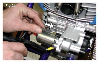
**3.8.2** CONNECT THE TERMINAL OF THE IGNITION STATOR TO THE H.T. COIL (SEE FIG.25).
