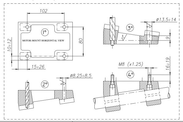
3.3.2 INSTALL THE MOTOR-MOUNT. MAKE SURE TO USE M8 ALLEN SCREWS WITH A LENGTH SUCH AS TO ENGAGE, IN THE CRANKCASE, A THREADED PORTION LENGHT OF 16÷19mm (THE SCREW MUST PROTRUDE FROM THE PLATE, FOR (16÷19mm) (SEE FIG. 4 AND DRAW.)
