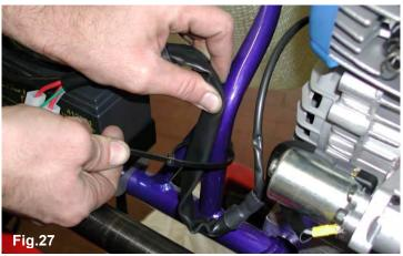
3.8.5 FIX THE BATTERY AND HARNESS TERMINALS BY MEANS OF THE STRAP (SEE FIG.28).
