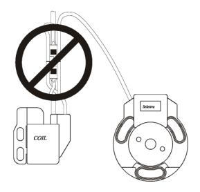
Always make sure to ground the coil. Failure install ground strap will cause the coil short circuit and be damaged beyond repair.
