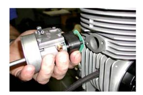
Connect the plastic tube between the pressure pulse on the carburetor and on the fitting on the crankcase  $\rightarrow$
