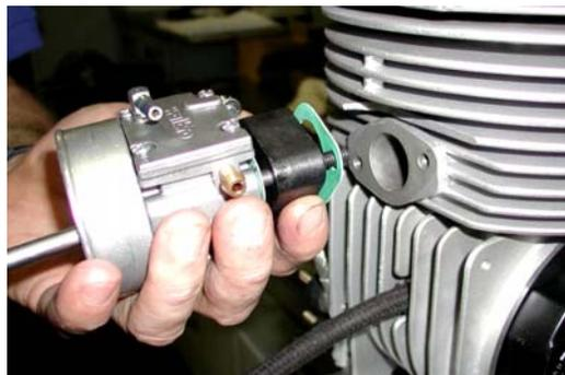
Connect the plastic tube between the pressure pulse on the carburetor and on the fitting on the crankcase →
