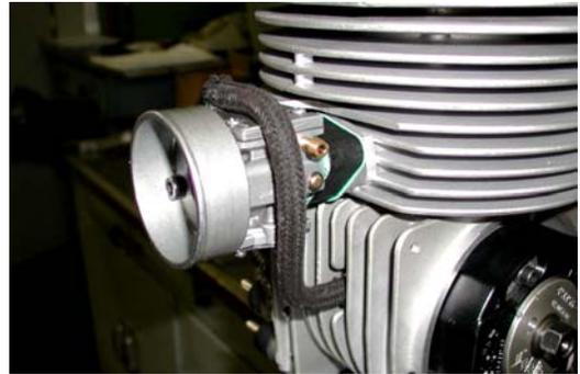
← Connect the throttle cable to the carburetor and use a spring to improve the quick response of the carb throttle
