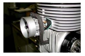
$\leftarrow$  Connect the throttle cable to the carburetor and use a spring to improve the quick response of the carb throttle
