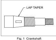
and the crankshaft with fine lapping compound. Clean off the lapping compound before installation.
